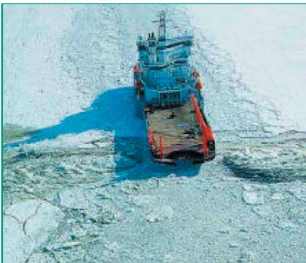
Lateral mixing feature of icebreaker, Fennica. Thrusters clearing channel. (Aker Finnyards)
